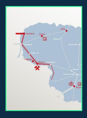
Reinforced Jurbarkas-Bitėnai overhead line will allow to integrate 700MW wind energy
