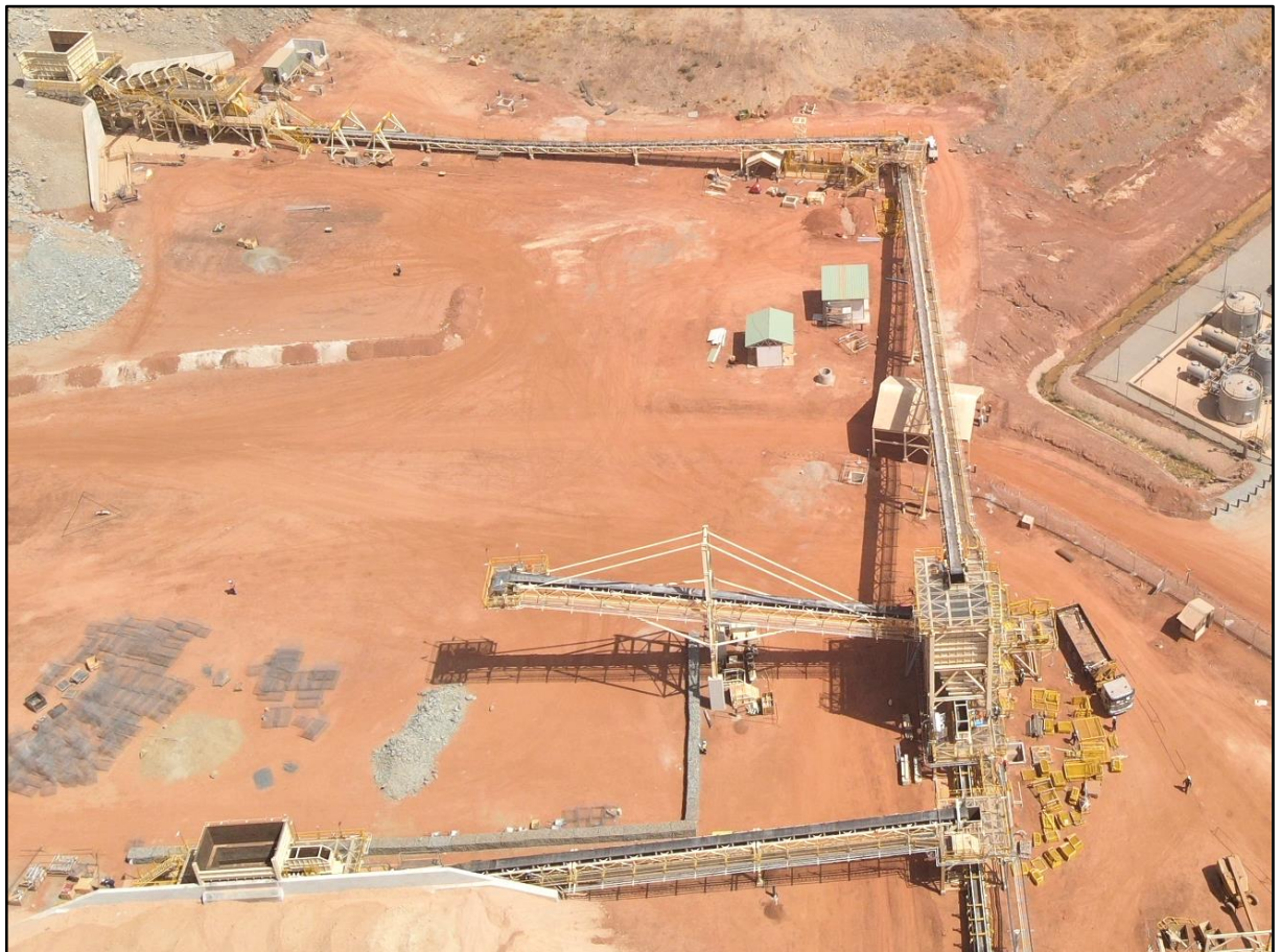
Figure 2: Crushing circuit construction is complete and wet commissioning of the primary jaw crusher is underway
