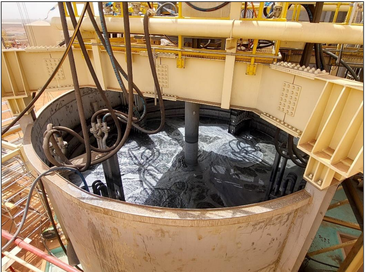
Figure 6: BIOX® inoculum currently active in the back-up reactor
