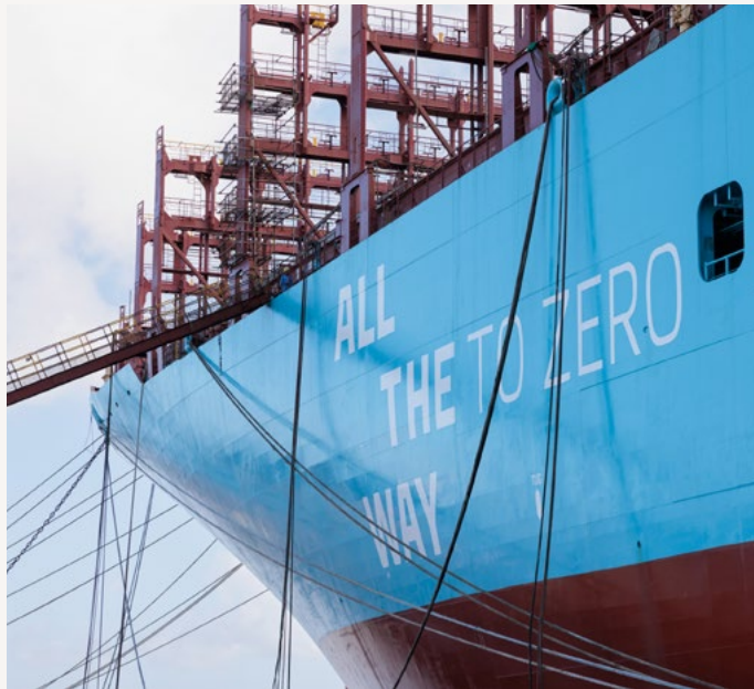
In an industry first, the Maersk Halifax was retrofitted as a dual-fuel methanol vessel at the Zhoushan Xinya Shipyard, China in 2024.
