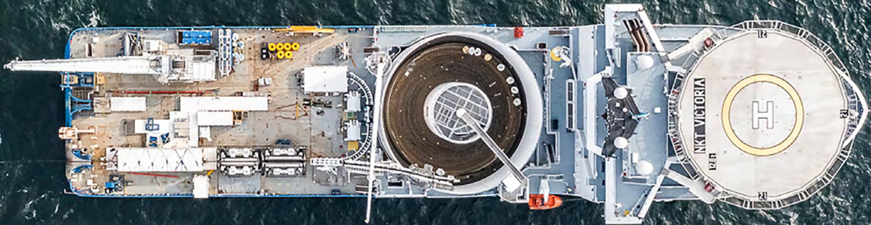
NKT Victoria is one of the world's most advanced and fuel-efficient cable-laying vessels. The two turntables on the vessel have a combined capacity of 9,000 tonnes high-voltage power cables.
