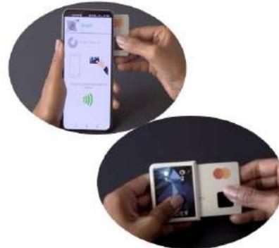
Using one of our proprietary solutions, a user can complete the enrolment process in less than a minute, following simple instructions. Enrolment is completed entirely within the biometric smart card and, importantly, the encrypted fingerprint template is immediately stored only on the card, never in the cloud or on any connected device such as a smart phone or PC.
