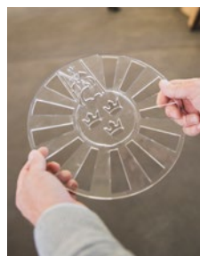
Laser cutting of logo in clear PMMA (acrylic). Opido can machine PMMA up to 30mm thick in two laser cutting machines, 2x3m in size.
