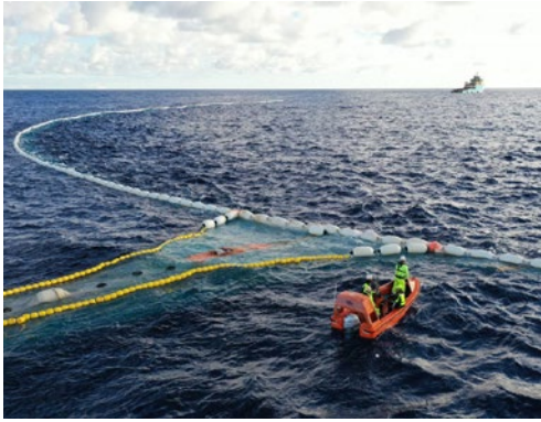
Fenders from Dan-Hill-Plast A/S are used for buoyancy of landing nets in connection with the collection of plastic waste in the ocean. Source: The Ocean Cleanup.
