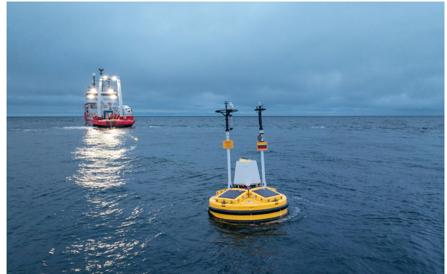
Wind and meteorological measurements for an offshore wind project in the Baltic Sea
