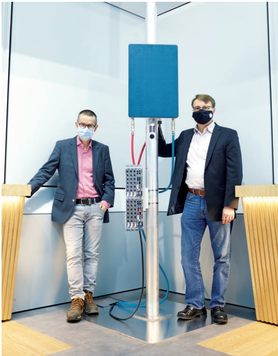
◀ Our ground-breaking liquid-cooled 5G base station system offers 90% lower cooling system energy consumption and 80% lower base station CO 2 emissions.
