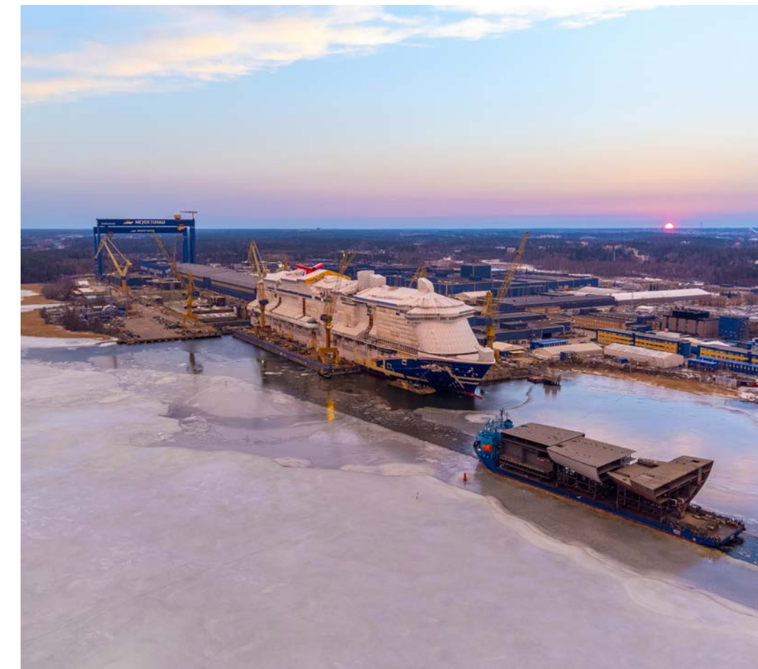
Open deck carrier Meri carrying ship blocks, arriving at Turku Shipyard, Meyer Turku.
