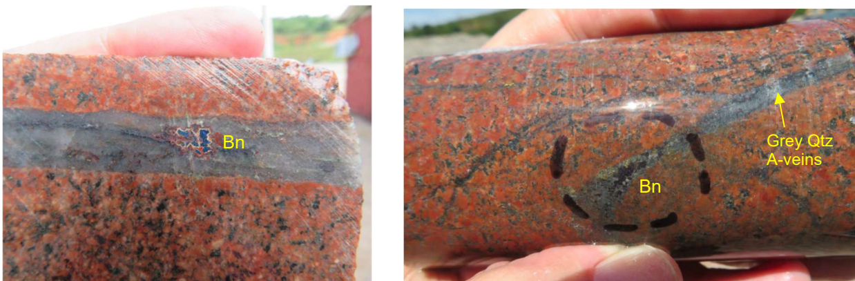
Figure 4: Photographs illustrating bornite mineralisation within A-veins. Abbreviations: Qtz – Quartz, Bn – Bornite
