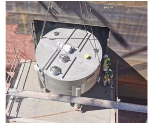
Pictures show Scanship equipment being retrofitting on Carnival Dream
