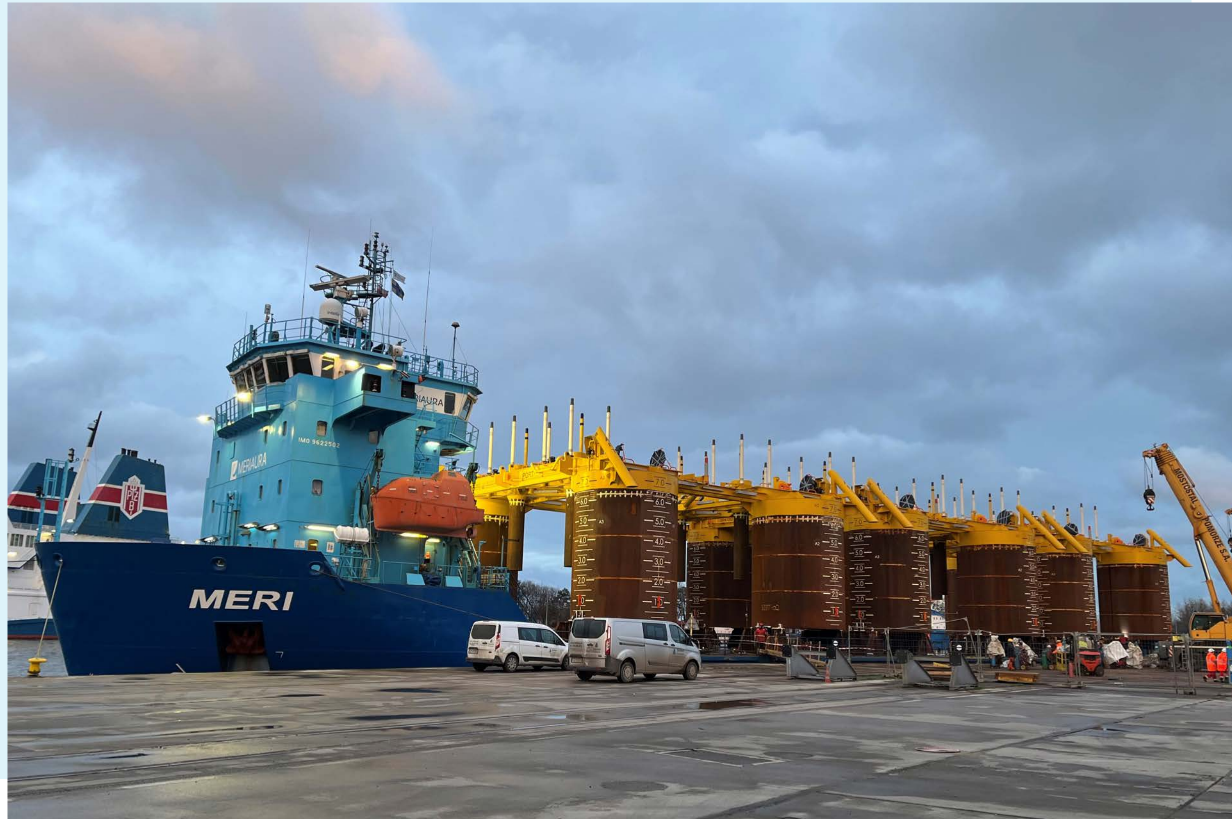
Deck cargo carrier 'Meri' loaded offshore structures in Gdansk for Subsea 7.
