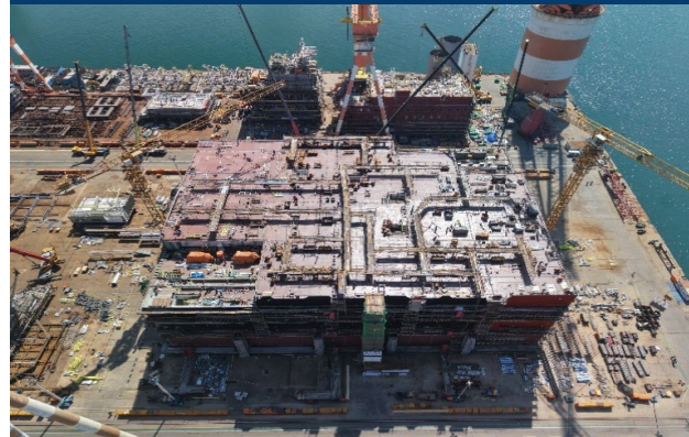
Midship fabrication status – all blocks installed
