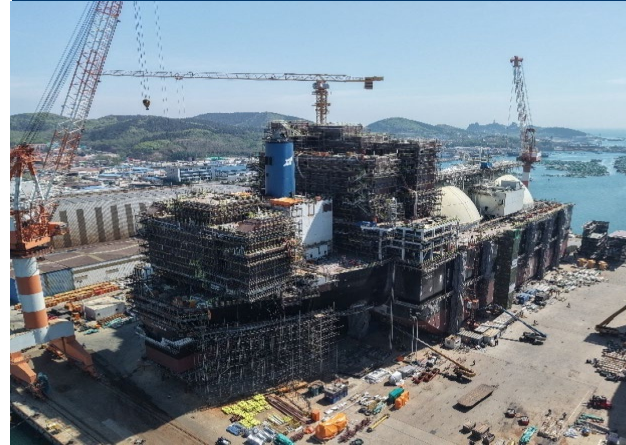
Midship fabrication status – all blocks installed
