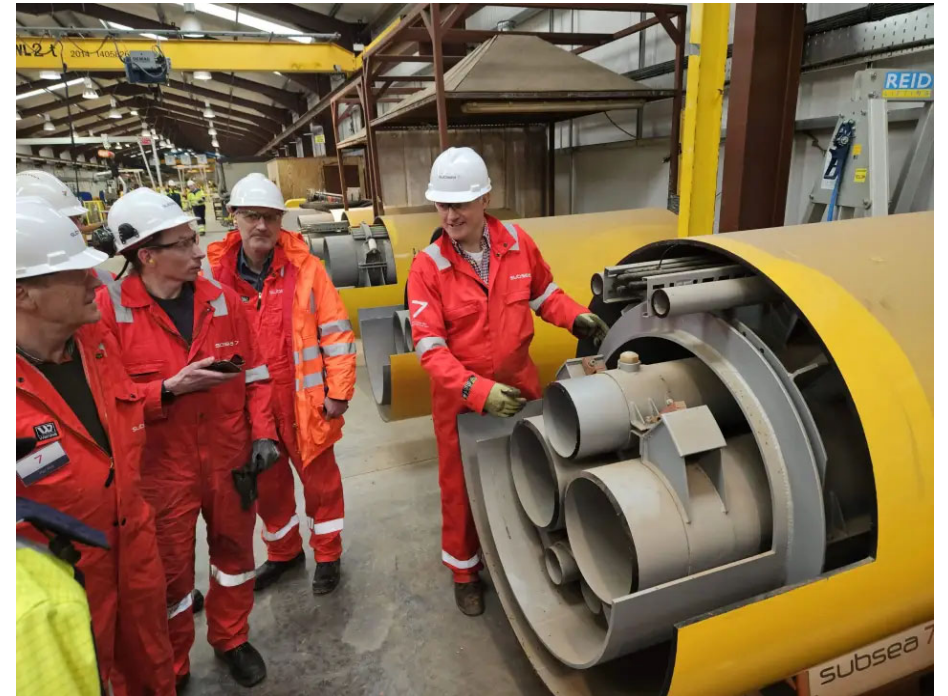
A pipeline bundle cross section at Wick
