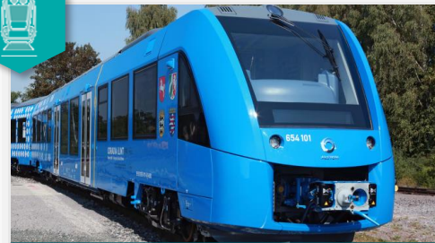
World's 1st hydrogen-powered regional train Coradia iLint from Alstom, Germany (Photo: Alstom)
