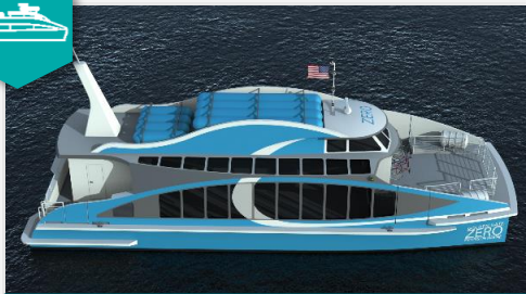
1st hydrogen vessel in the U.S; 70 ft hybrid hydrogen fuel cell battery catamaran to be sailing (Photo: Golden Gate Zero Emission Marine)
