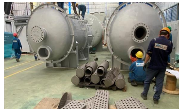
Steam drums for Heat Recovery Steam Generators (Kanfa)
