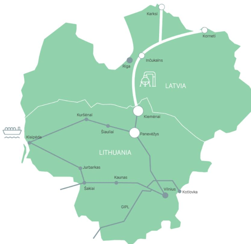
The project will increase the capacity of the Kiemėnai gas metering station and reconstruct the pipeline to the Panevėžys gas compressor station on the Lithuanian side, while in Latvia the project will cover reconstruction of the main gas pipeline to increase the maximum operating pressure from 40 to 50 bar.
