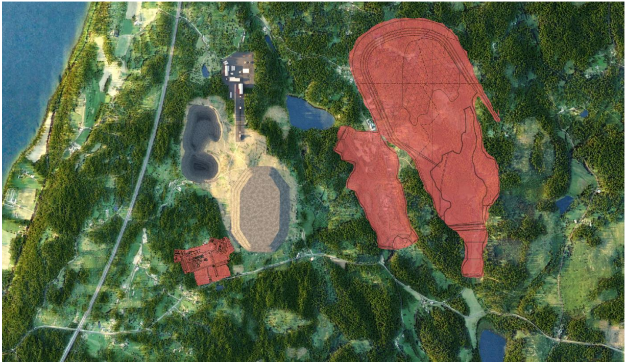
Figure 1 – Graphical illustration of Norra Karr On-site open pit, waste rock facility and physical beneficiation plant in comparison to 2015 PFS infrastructure and tailings dam (in red)
