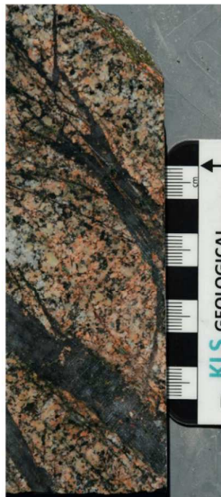
Qz-Mgt-Cpy [Kspar-Bt2] vein 23MT006 – 210.8m
