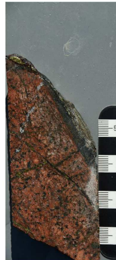
Immature Supergene Enrichment Cpy → Cv-Glassy limonite 23MT007 – 248.6m
