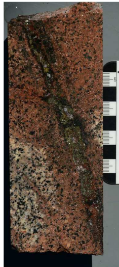
Hematite-Kspar Alteration 23MT004 – 23m
