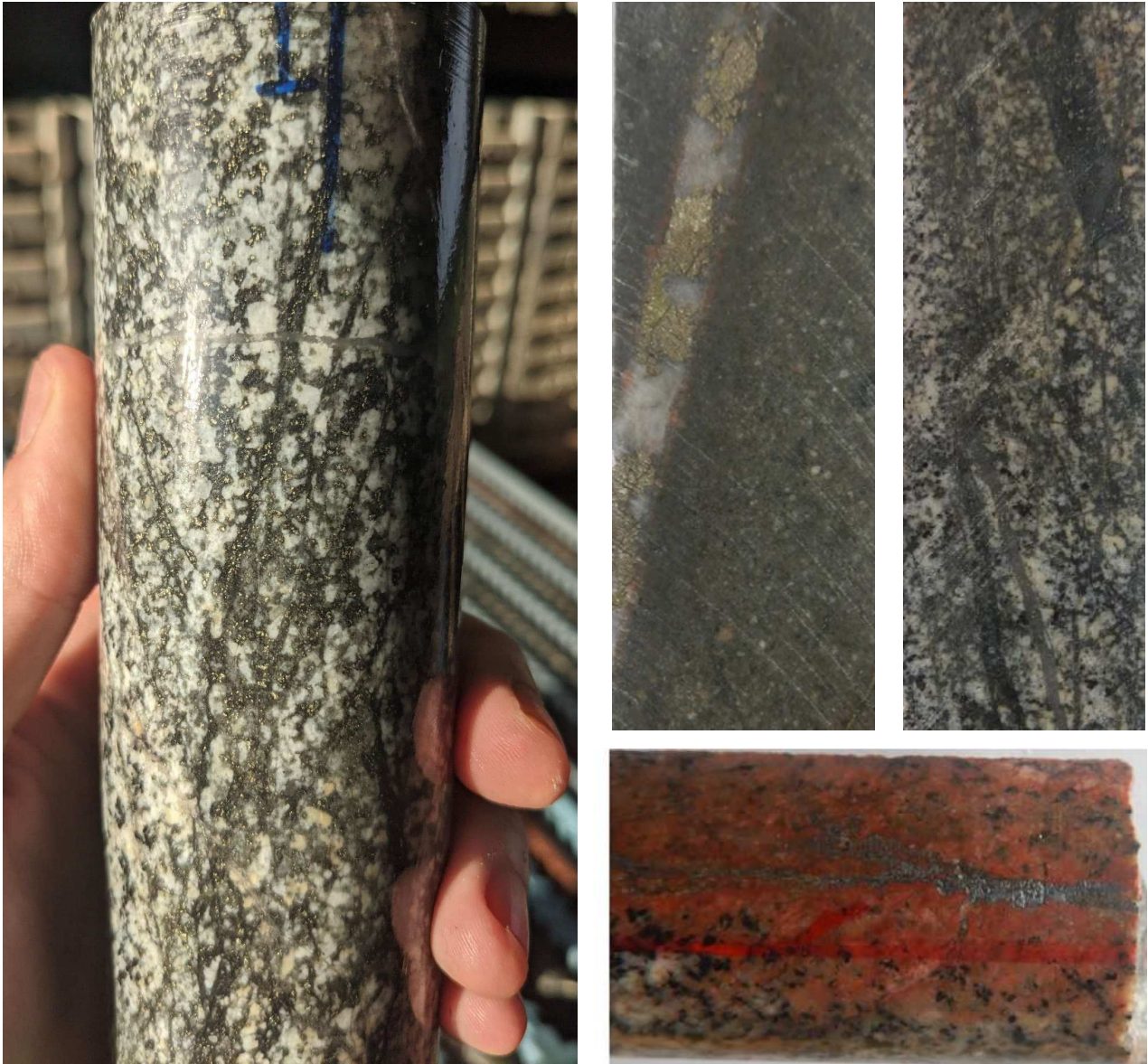
Figure 8: Images of Matilda drill core showing porphyritic textures, potassic alteration and veining and stockworking with significant sulphide (pyrite, chalcopyrite and molybdenite) content
