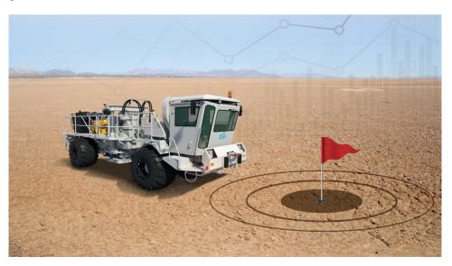
Sercel's Vibrator Auto-Guidance solution optimizes the Nomad's travel time to the next vibrating point (image courtesy of Sercel).
