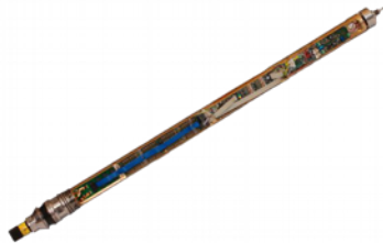
Ultrasound camera for Down Hole inspection for Tecwel (Archer)
