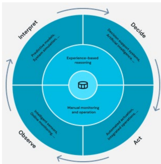
Figure 11 - Precision Fish farming: A cyclical representation where operational processes are considered to consist of four phases: Observe, Interpret, Decide and Act. The inner cycle
