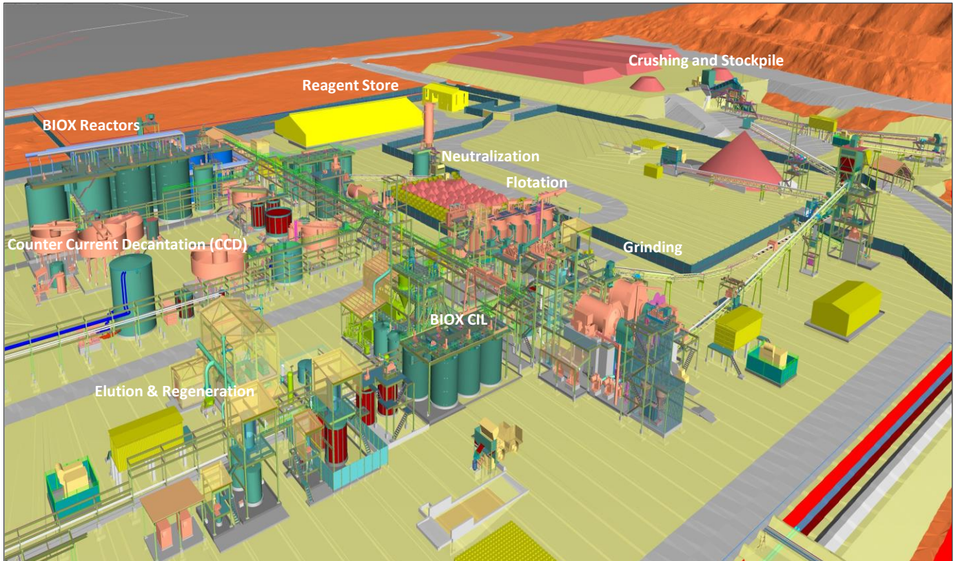
Figure 3: Sabodala-Massawa Expansion Project Site Layout
