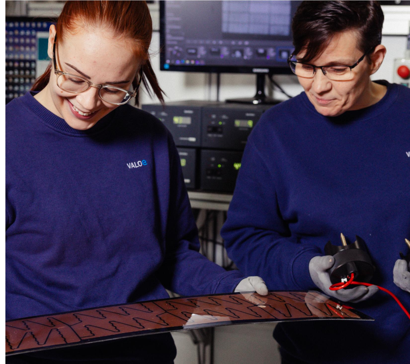
Valoe designs a separate "motherboard" for each panel. This ensures that the back contact module has the best possible efficiency optimised for its shape and surface area. Cell efficiency is essential in modules that are often very small. Valoe's IBC cells are among the most efficient on the market.
