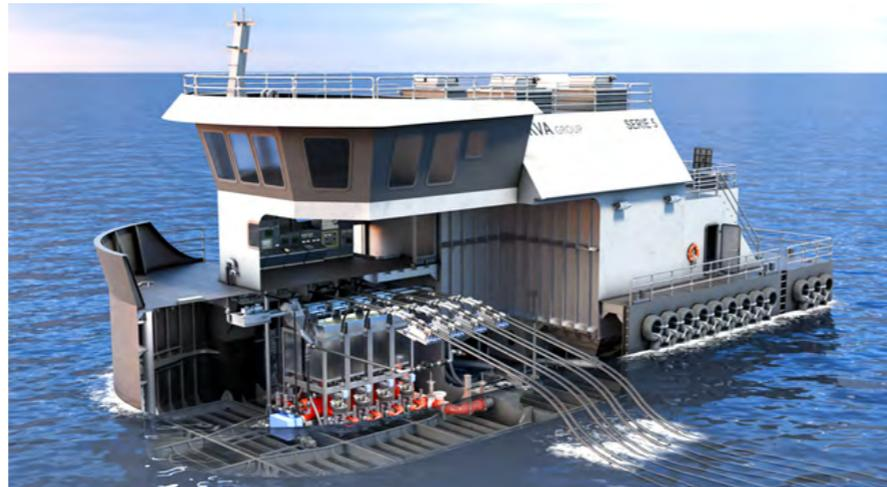
Figure 24 - Barge with waterborne feeding system
