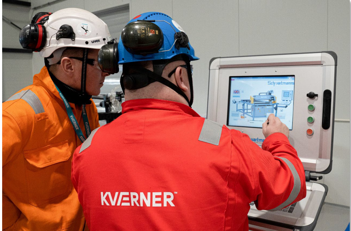
Photo from new digitalised insulation manufacturing line. Insulation boxes can now be manufactured automatically, versus traditional process with all-manual measuring, drawing, manufacturing.
