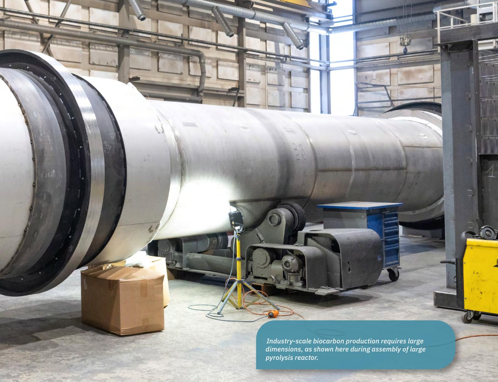
*Industry-scale biocarbon production requires large dimensions, as shown here during assembly of large pyrolysis reactor.*
