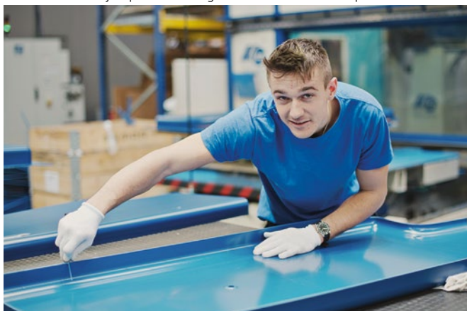
Andrezej Filipiak deburring a vacuum-formed component.
