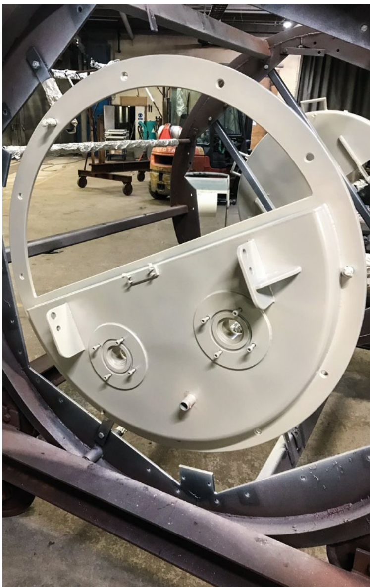
Tank top coated with food grade Accotron BFA.
