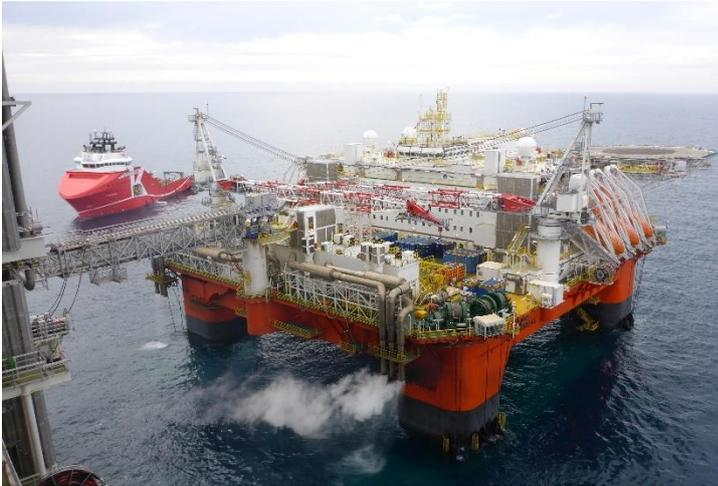
Safe Boreas was built at Jurong Shipyard in Singapore to the GVA 3000E design utilising GVA's extensive semi-submersible design experience. The vessel is designed for worldwide operations in the harshest offshore environments including the North Sea, and can operate both in DP and anchored mode, providing maximum cost efficiency and flexibility.
