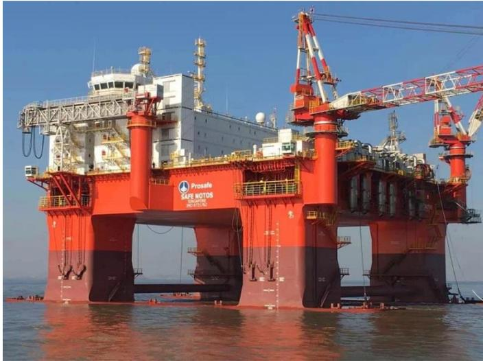
Safe Notos was built at Cosco to an enhanced Gusto MSC's Ocean 500 design incorporating DP3 station keeping systems, 10-point chain mooring and variable draft operations in the harshest offshore environments, excluding Norway.
