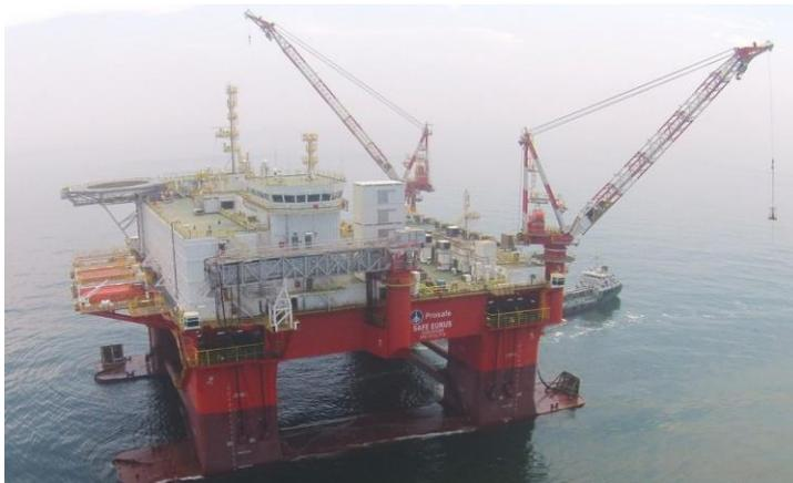
Safe Eurus is a technologically advanced and flexible DP3 semi-submersible ASV designed for worldwide operations, excluding Norway.
