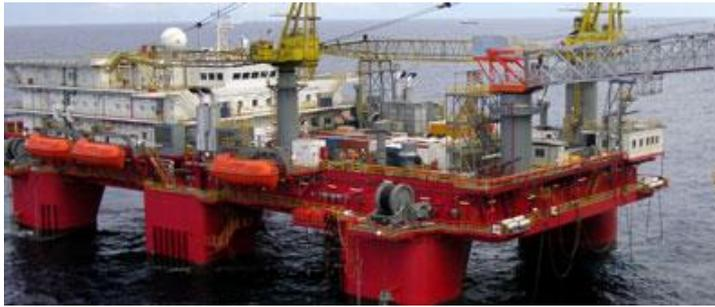
Safe Concordia is a self-propelled semi-submersible accommodation and service vessel of twin hull configuration, capable of operating in benign to moderately harsh environments.
