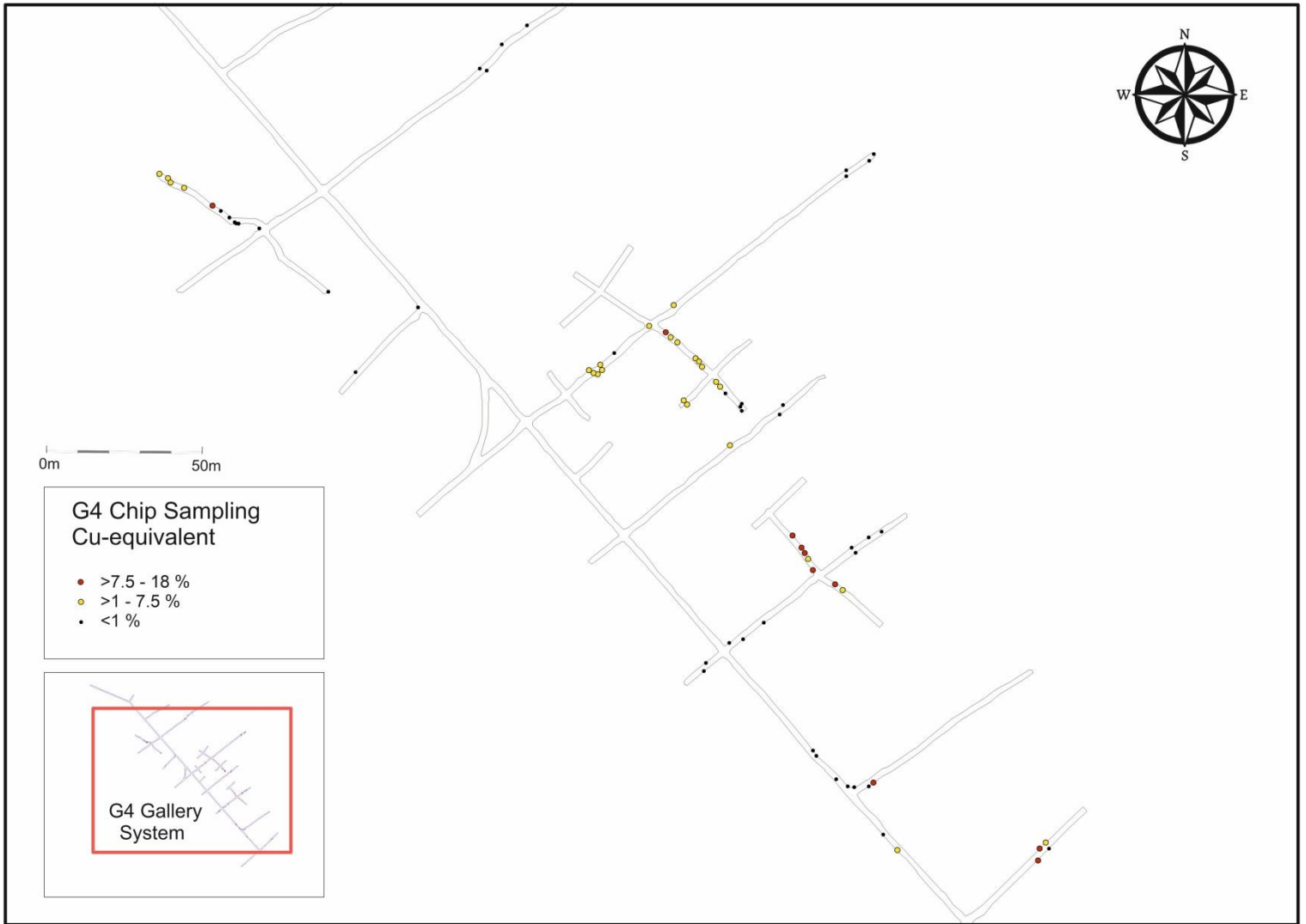
Figure 3: Location of chip samples in G4 on mineralized NW-SE structures. Zoom in for more detail.
