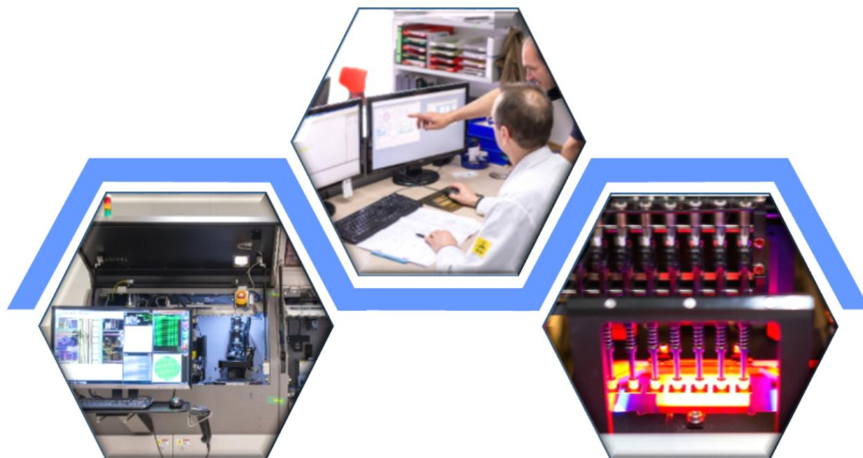
**Wafer & component testing** is the heart of the production function within RoodMicrotec, which means running an automated test floor 24 hour per day, 7 days per week. In this area, we perform the services of wafer testing, component testing, component programming, straightening, scanning and tape & reel of the semiconductor devices.
