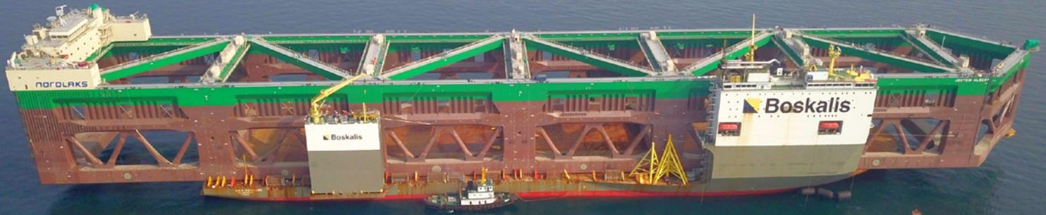
The BOKA Vanguard transporting a fish farm measuring 385 by 60 meters making it the largest cargo ever transported by vessel
