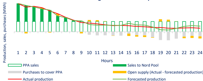
Example of transactions in a wind energy portfolio with baseload PPAs during a theoretical 24h period
